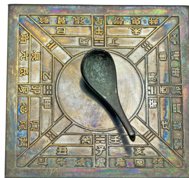
FIGURE 2.6.2b: The magnetic compass has been used by navigators for about a thousand years. By taking bearings of visible objects with a compass, navigators can work out the position of their ship.
