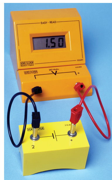
FIGURE 2.6.12d: A voltmeter connected to measure the voltage of a cell
