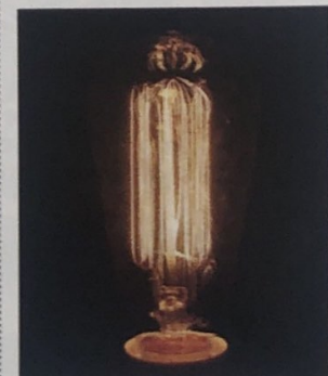
FIGURE 2.6.14b: An early tungsten filament light bulb
