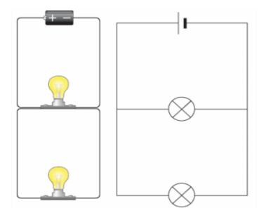
An example of a parallel circuit.
