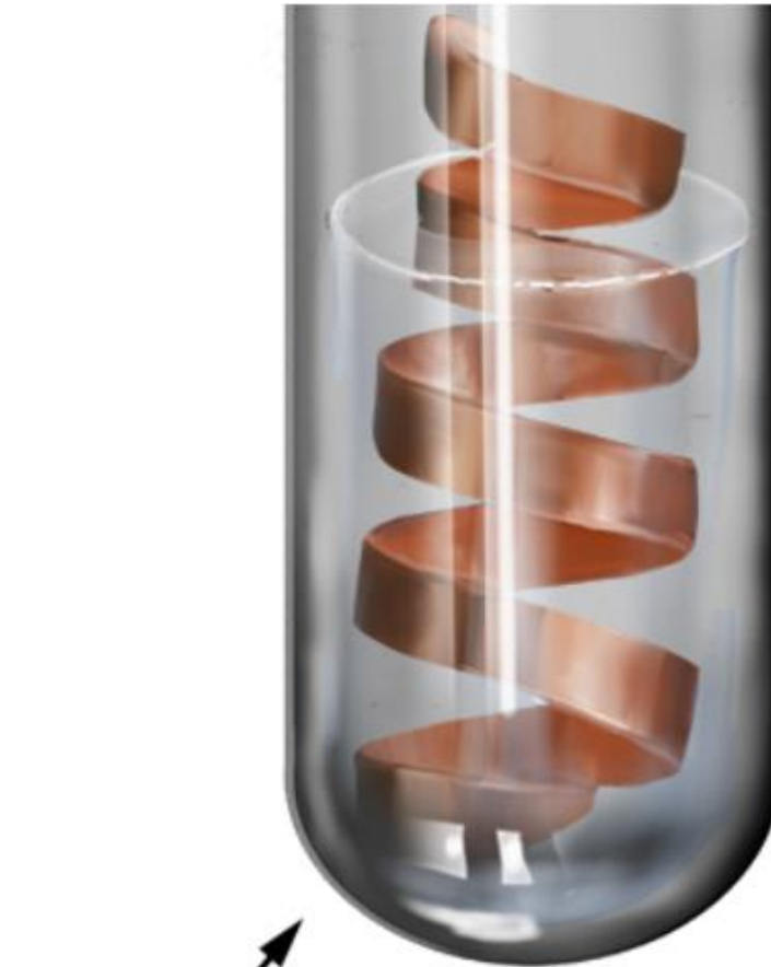
Copper in hydrochloric acid
