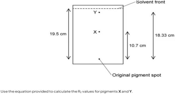
$R_{f} = \frac{Distance moved by pigment}{Distance moved by solvent}$
