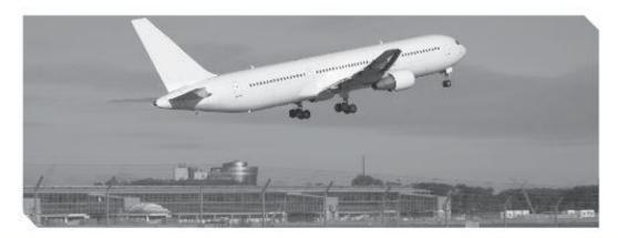
Thrust force acts on the plane to make it move forward, Air resistance acts on the opposite direction of motion, Gravity acts downward while the wings apply an upward force to make it fly upward.
