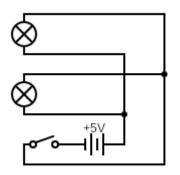
• There are two LEDs that give off 1400 L each, connected in parallel and activated by a switch. There are also five sockets. It is all connected with twenty-three metres of wire.
