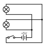
• There are two LEDs that give off 1400 L each, connected in parallel and activated by a switch. There are also two sockets. It is all connected with fifteen metres of wire.
