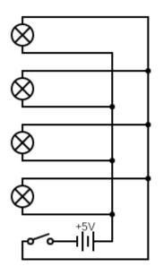
• There are four LEDs that give off 800 L each, connected in parallel and activated by a switch. There are also four sockets. It is all connected with twenty-four metres of wire.
