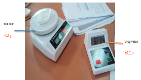
Figure 3.1 and 3.2: Some of the apparatus labeled (these pictures were taken at the end of the experiment)
