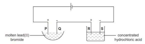
At which of the electrodes is a Group VII element produced?
