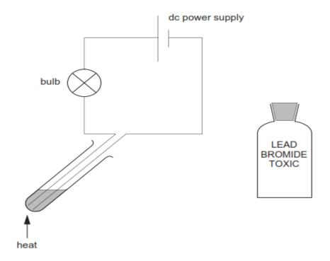
The lead bromide was heated until molten. A brown gas was given off.
